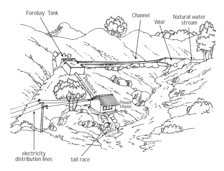
Water from the river is channelled through a settling basin, which helps to remove sediments that could harm the turbine. The water then flows into the forebay tank where it is directed downhill through a pipe called a penstock. When the water reaches the bottom, it drives a specially designed turbine to produce the electricity. (Source:'Micro-hydro power: the basics', Practical Action, available at http://practicalaction.org/?id=micro\_hydro\_faq)
